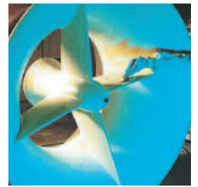
Pump Bellmouth receiving erosion, abrasion and corrosion resistant Weir protect lining system.
