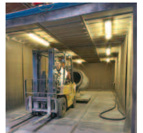
Multi-stage borehole pump bowls receiving potable water approved glass flake lining.
