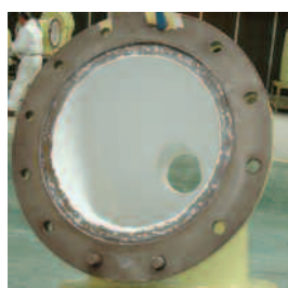
Typical unlined coastal power station CW pipework.
