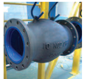
Glass flake lined ECW pipework destined for nuclear power station.
