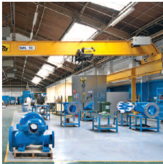
Epoxy powder coated valves and pumps.
