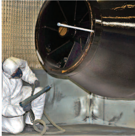
Large pump bowl/chamber receiving abrasion resistant powder coating.
