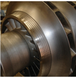
Eye seal diameter following repair.
