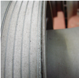
Erosion in first stage eye seal diameter.
