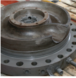
The compound curves of the discharge volute were achieved using 5-axis milling techniques.
