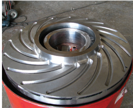
Hub and shroud weld prep.
