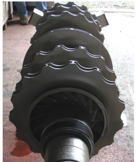
Figure 1. Scalloped impeller on original rotor.
