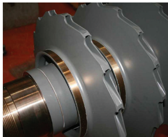
Figure 8. Teflon coated rotor.
