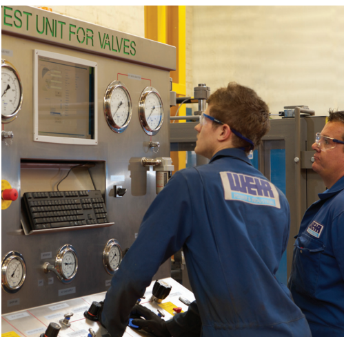
Valve, controls and actuators are tested simultaneously on Weir's state-of-the-art testing equipment.
