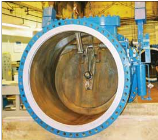
Compressor Check Valve with Oil Dashpot
