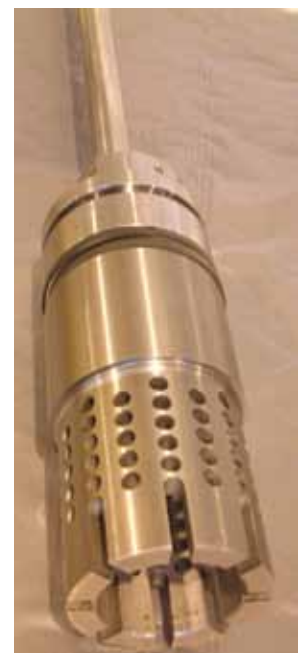
Tungsten carbide plug head for erosion control
