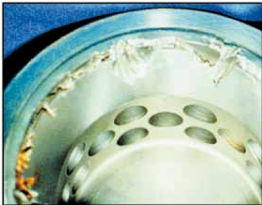
Potential damage through incorrect trim selection
