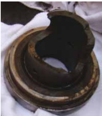
Example of failure of externally sleeved Choke
