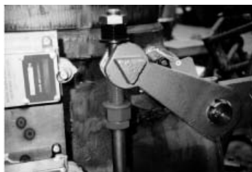
Incorrect Setup: more than 1/8" between bottom Flange Nut Face and Lower Arm.
