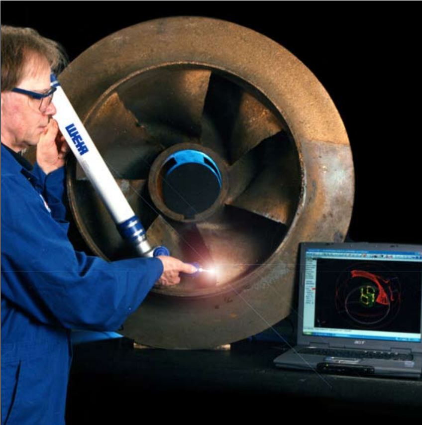
Coordinate measuring machine used to produce detailed drawings to enable reverse engineering of components
