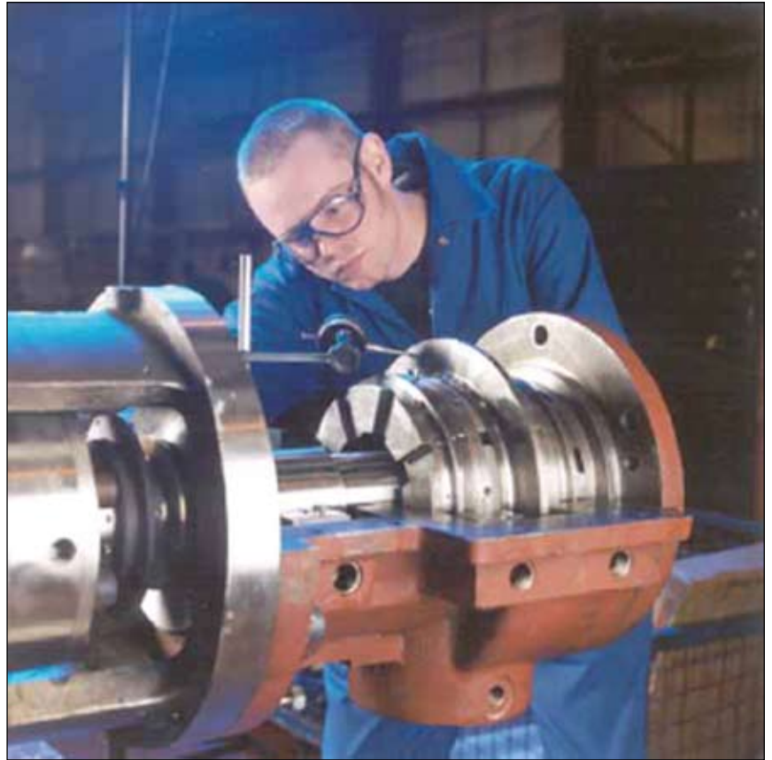
Final pump alignment after overhaul being carried out prior to shipping to offshore platform for installation
