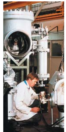
Above: Atwood & Morrill Bled Steam Non-return Valve for use in power generation.
