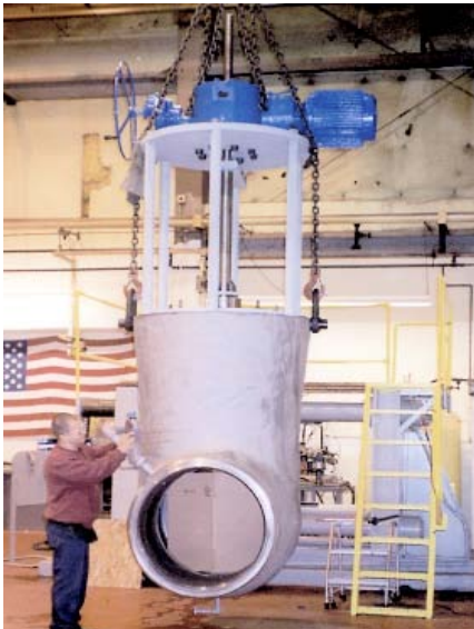
36" Class 405 SPL INT Parallel Slide Gate Valve WT – 25,300 lbs. 15 ½ Ft. Tall
