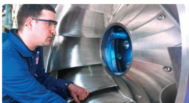
Inspection of Francis turbine runner for hydro power station
